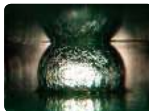
PBGA – scaling: insufficient heat
