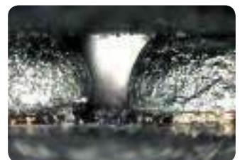
PBGA – scaling: insufficient heat
