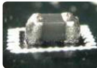
0402: bulbous solder joint
