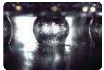
PBGA – cold joint: insufficient heat
