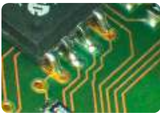
Lead-free assembly: non-wetting
