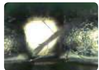
BGA: contamination (fibre)
