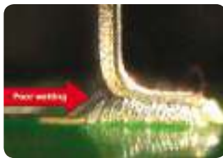
PQFP – interior fillet: poor wetting
