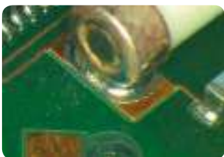
Lead-free assembly: non-wetting
