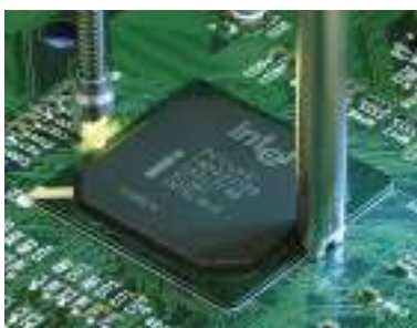
ERSASCOPE 1: fixed optics for BGAs
