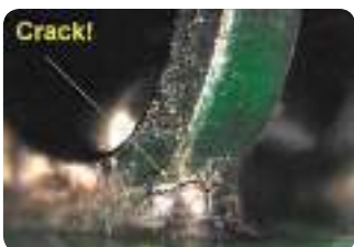
Lead-free PLCC: micro crack
