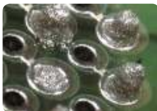
BGA – paste print: insufficient solder
