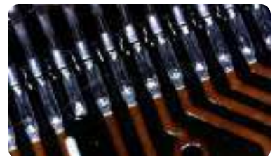
QFP solder joints – taken with the Erska MOBILE SCOPE MACROZOOM optical head
